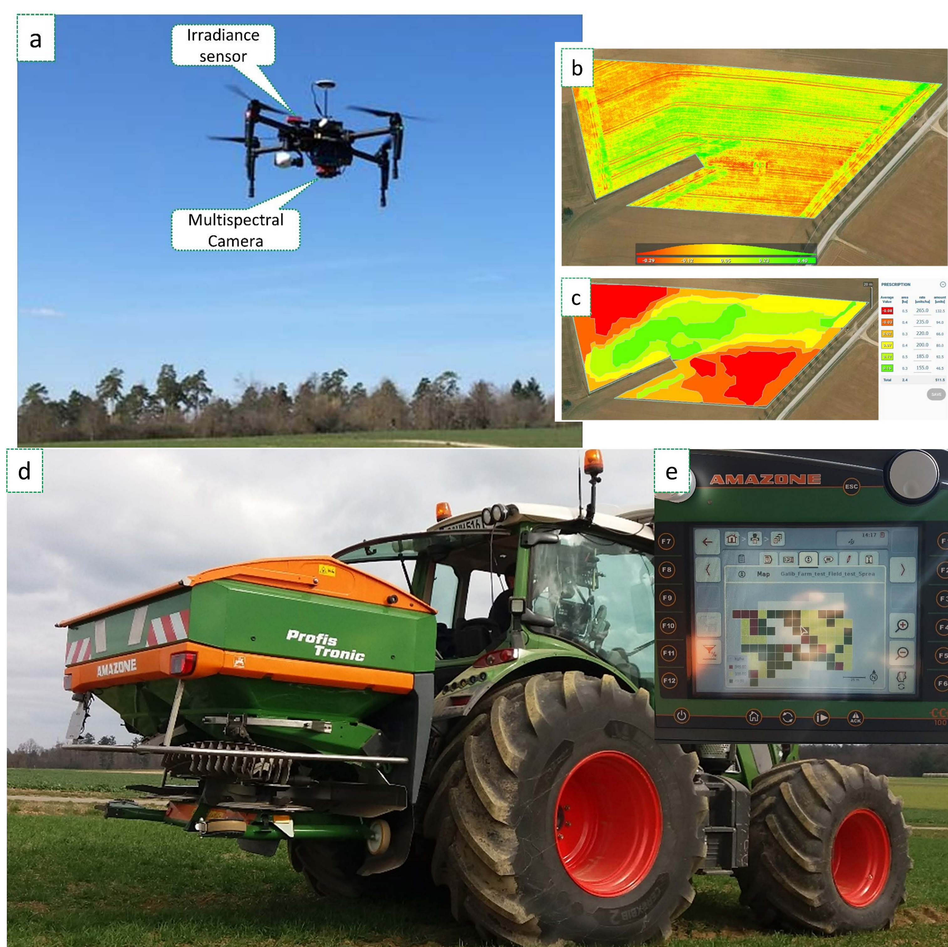
a – Acquisition of airborne data, b – NDVI map, c – VRA prescription map, d – Utilised Amazone ZA-V spreader, e – Implemented VRA prescription map on VT
