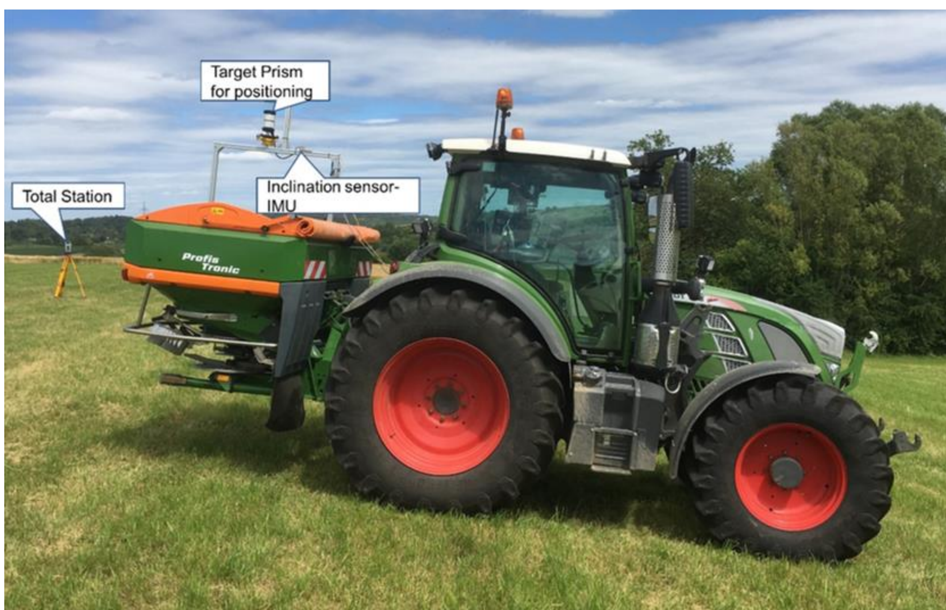
Figure 1: A centrifugal spreader designed with high accuracy positioning sensors for performing VRA.
